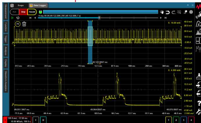
Figure 19. CX3300 can read and playback from the storage for deep analysis similar to the scope
