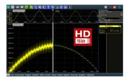
The Rohde & Schwarz RTx-K31software option provides essential measurement functions for analyzing power electronics, including inrush current, output spectrum and safe operating area. A measurement wizard with detailed instructions guides the user through the test setup. The oscilloscope configures itself automatically and delivers quick results. Optimal display configuration for each task.
