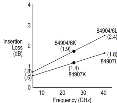
Figure 1. Insertion loss
