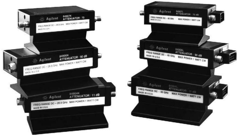
This latest design evolution sets new standards for size and performance. High attenuation accuracy and low SWR are achieved through the use of miniature thin-film attenuation cards composed of high-stability tantalum nitride film on a sapphire substrate. Insertion loss performance is outstanding, with less than 2 dB of loss at 26.5 GHz and only 2.4 dB at 40 GHz (figure 1).
