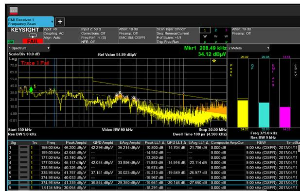
Figure 2. Conducted emissions with delta to limit
