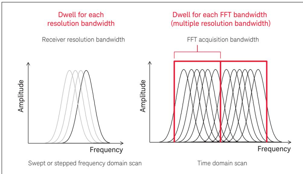
Figure 7. Comparison of resolution and FFT acquisition bandwidths
