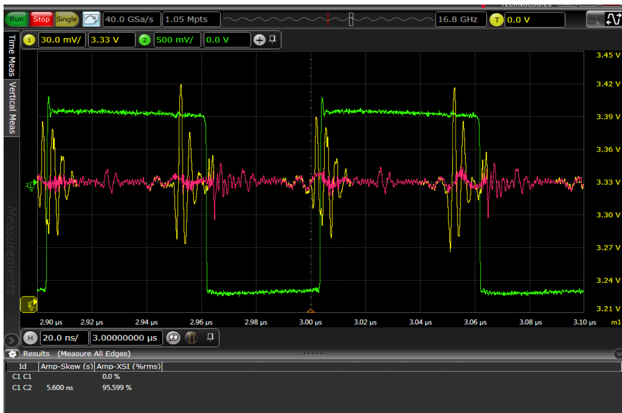
Figure 14. Example of a power supply being treated as a victim. Victim waveform (yellow), aggressor (green) and crosstalk-removed waveform (red).
