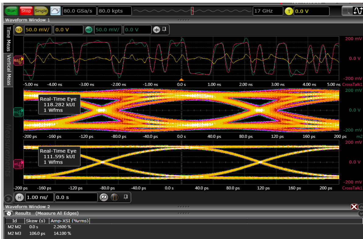
Figure 10. Before and after view of a victim waveform with FEXT. The top plot shows the victim waveform in green, the aggressor in orange, and the crosstalk removed waveform in red. The middle plot is the eye diagram of the victim with the bulging indicative of FEXT, and the bottom plot is the eye diagram of the victim after removing crosstalk.
