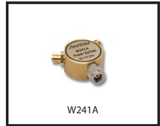
These microwave power splitters are symmetrical, two-resistor designs that can be used in applications where signals from DC to 110 GHz must be accurately divided for ratio measurements. They provide excellent flatness and effective output SWR.
