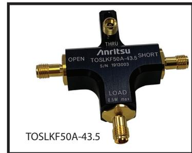
The TOSL series Thru/Open/Short/Load calibration kits have been designed to provide superior measurement results when used with precision instruments. It is designed for use in both field and lab environments. TOSL series Thru/Open/Short/Load comes in both N(male and female) and K(male and female) connector configurations. The K and Extended-K connectors are compatible with 3.5 mm and SMA connectors.
