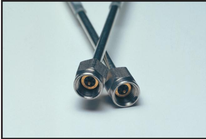
The K Connector® is a precision coaxial connector system that operates up to 40 GHz. It is compatible with SMA, WSMA, and 3.5 mm connectors. It is well suited for applications in components, systems, or instrumentation.
