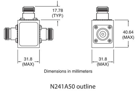
These RF power splitters are symmetrical, two resistor designs that can be used in applications where signals from DC to 3000 MHz must be accurately divided for ratio measurements. They are available in 50 Ω and provide excellent flatness and effective output SWR.
