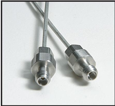
The W1 Connector® family is a complete coaxial connector system with mode-free performance to 110 GHz. Based on the 1.00 mm coaxial connector front side interface as specified by IEEE Std 287, the W1 Connector is well suited for high frequency applications ranging from components to systems and instrumentation.
