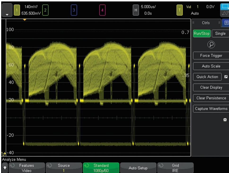
Figure 6. Triggering on 1080p HDTV.
