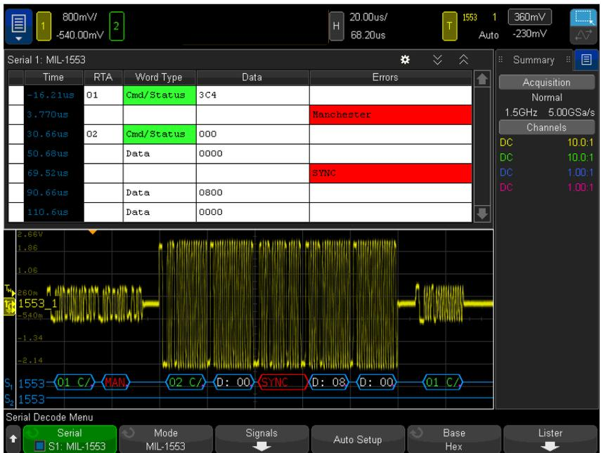
Figure 2. MIL-STD 1553 decode on an InfiniiVision X-Series oscilloscope.
