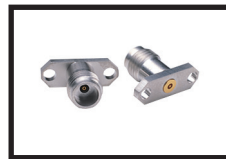
V103F-012 V Female Flange Launcher, two-hole for 0.30 mm glass bead pin, DC-65 GHz
