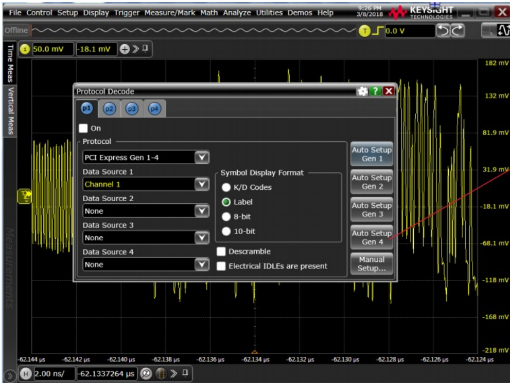
Figure 3. The auto-setup button for PCI Express. SAS and SATA have similar auto-setup buttons.
