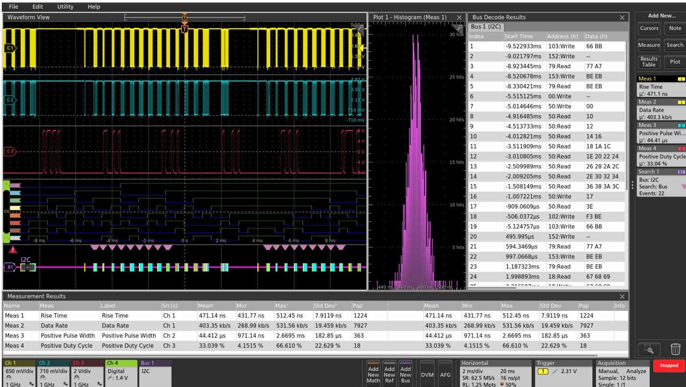
Viewing three analog channels, eight digital channels, a decoded serial bus waveform, decoded serial packet results table, four measurements, a measurement histogram, measurement results table with statistics and a search on serial bus events - simultaneously!
