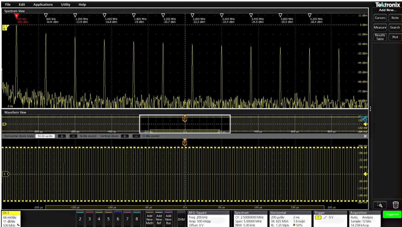
Spectrum Time gates the range of time where the FFT is being calculated. Represented by a small graphical rectangle in the time domain view, it can be positioned to provide time correlation with the time domain waveform. Perfect for conducting Mixed Domain Analysis. Up to 11 automated peak markers provide frequency and magnitude values of each peak. The Reference marker is always the highest peak shown and is indicated in red.
