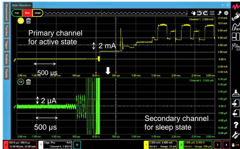
Figure 10. CX1102A measurement example
