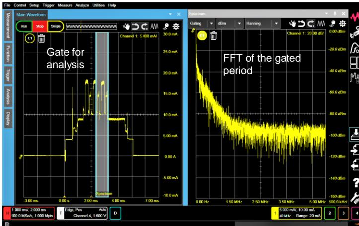
Frequency domain analysis (FFT) is available. You can focus on a specific period in the waveform by using the gating functions.
