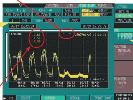
Dual screen display is possible for combinations such as voltage and current.
