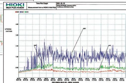
Print example: TIME PLOT screen (U-THD RMS fluctuation) printed on A4 paper
