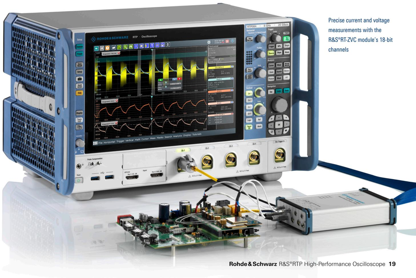
Precise current and voltage measurements with the R&S®RT-ZVC module's 18-bit channels
