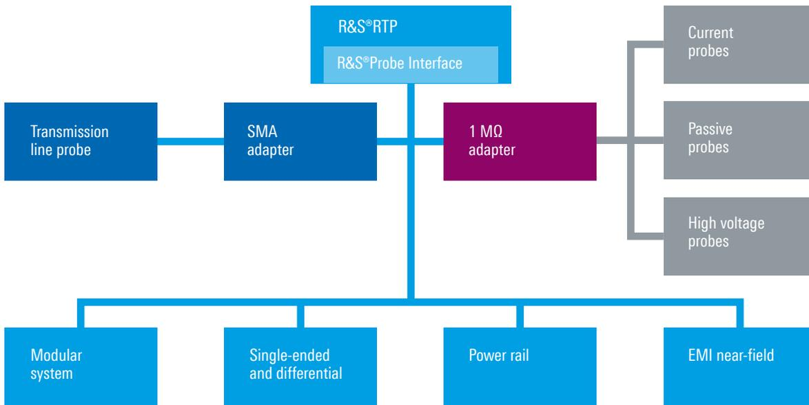
■ Probes which can be directly connected      ■ Probes which require R&S®RT-Z1M adapter
