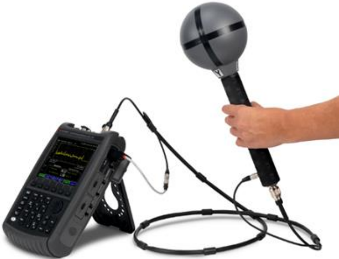
Figure 3. Connect the antenna to the analyzer
