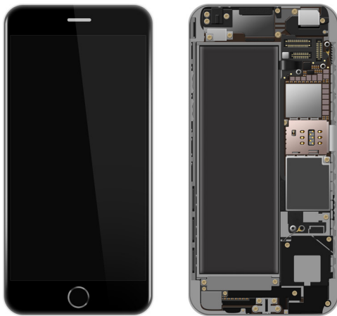
Figure 5: Modern smartphones are highly integrated systems with relatively few parts
