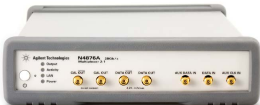
Figure 33. 28 Gb/s multiplexer 2:1 N4876A
