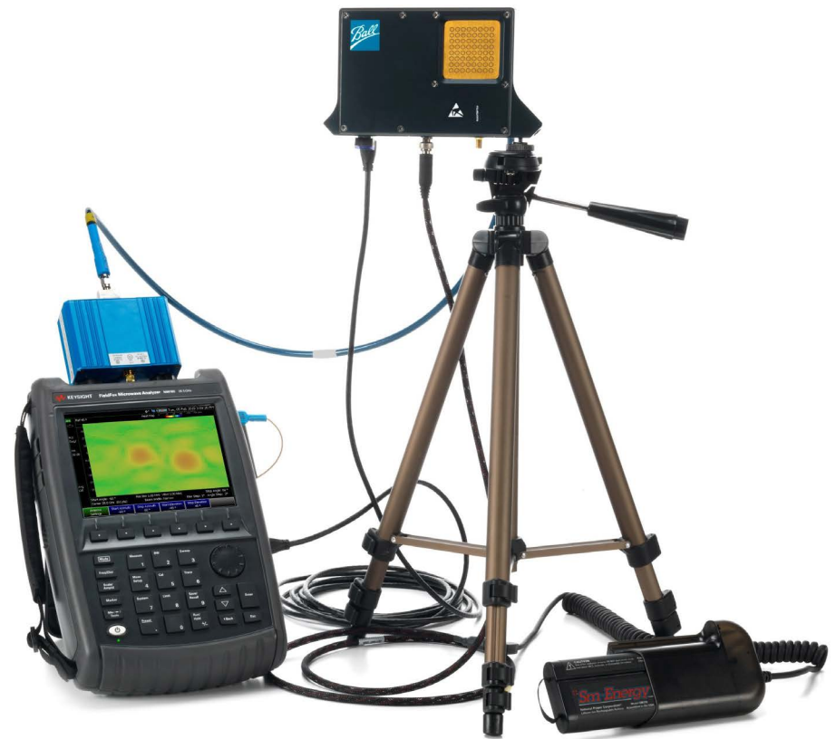
Figure 2. FieldFox and phased array antenna set up
