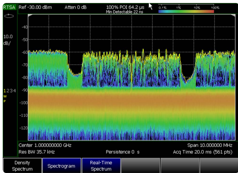
Figure 5. Beam sweep signals captured using FieldFox in RTSA mode
