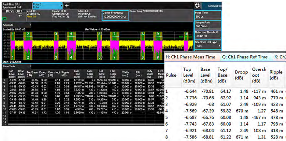
Figure 11. A graphical display of captured pulses (left) and a tabular summary of amplitude or power characteristics (right).
