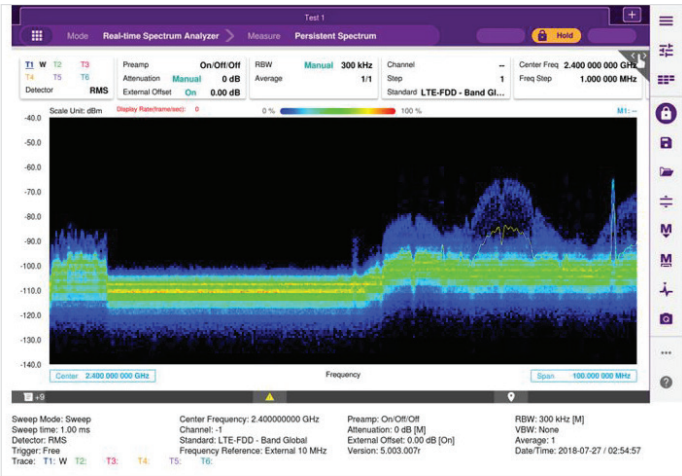
Fig 37: Persistent display showing interference signals in 2.4GHz band.
