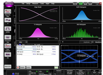
Figure 4. 32 Gb/s PRBS 211-1 showing 138 fs RJ_{rms} *
