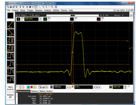
Figure 5. 100 ps pulse with 17 ps risetime.
