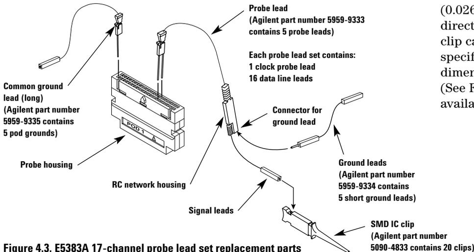
Figure 4.3. E5383A 17-channel probe lead set replacement parts
