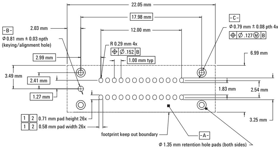
1. Must maintain a solder mask web between pads when traces are routed between the pads on the same layer. Soldermask may not encroach onto the pads within the pad dimension shown.
