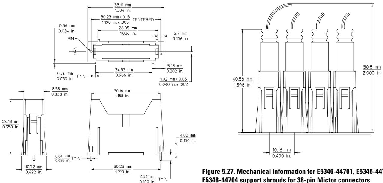
**Figure 5.27. Mechanical information for E5346-44701, E5346-44703, E5346-44704 support shrouds for 38-pin Mictor connectors**
