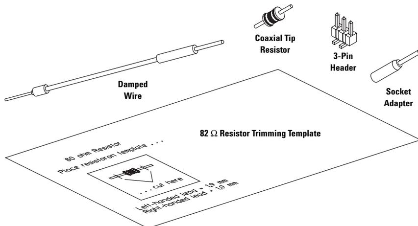
Figure 11.4. E5381A differential flying-lead probe set accessories
