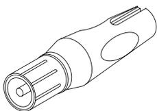
Figure 11.2. E9638A BNC to probe tip adapter
