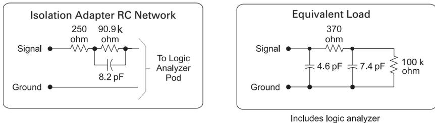
**Figure 7.3. Isolation adapter (01650-63203) and equivalent load**
