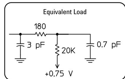
Figure 10.7. E5380A input equivalent load, including 38-pin connector
