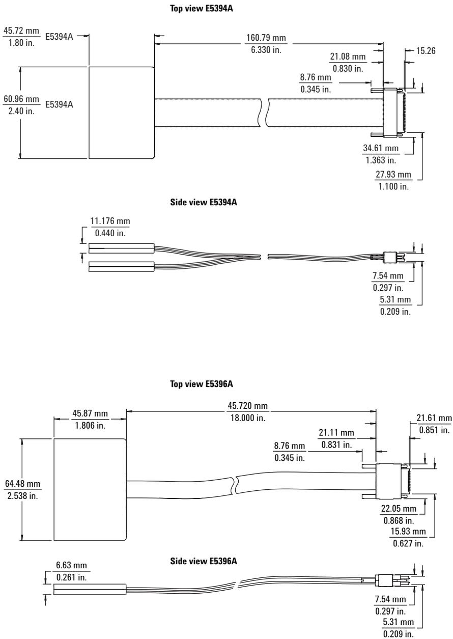
Figure 5.6. E5394A and E5396A soft touch probe dimensions
