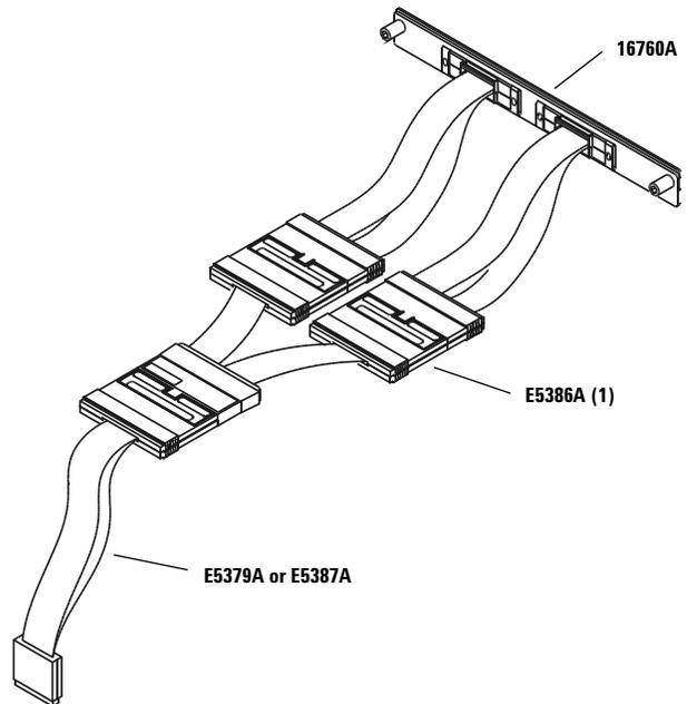
Figure 9.3. E5386A with E5379A, E5387A, or E5405A differential probe
