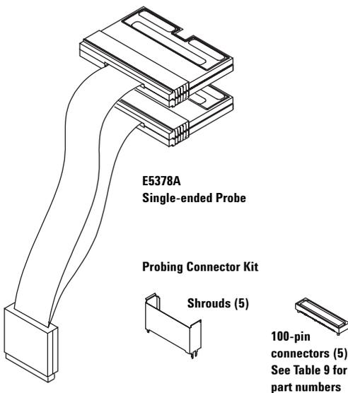
Figure 8.18. Agilent E5378A probe
