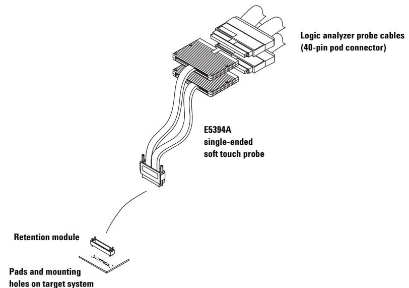
Figure 5.2. Agilent E5394A soft touch probe connection
