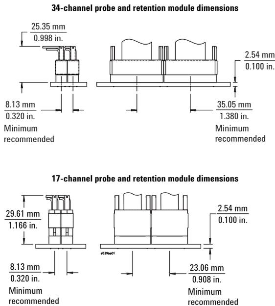
Figure 5.8. Side-by-side dimensions
