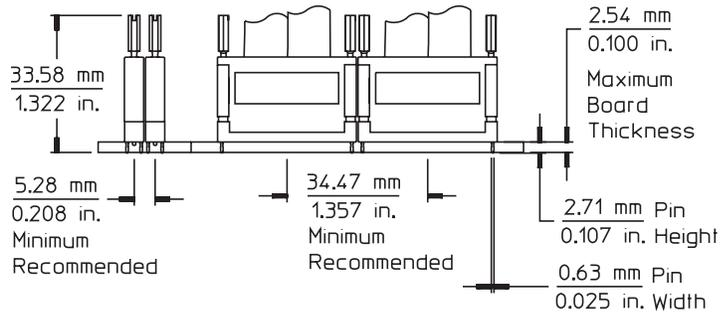
Figure 8.6. Pro Series soft touch side-by-side dimensions
