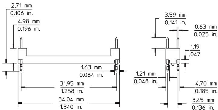
Figure 5.4. Pro Series soft touch retention module dimensions
