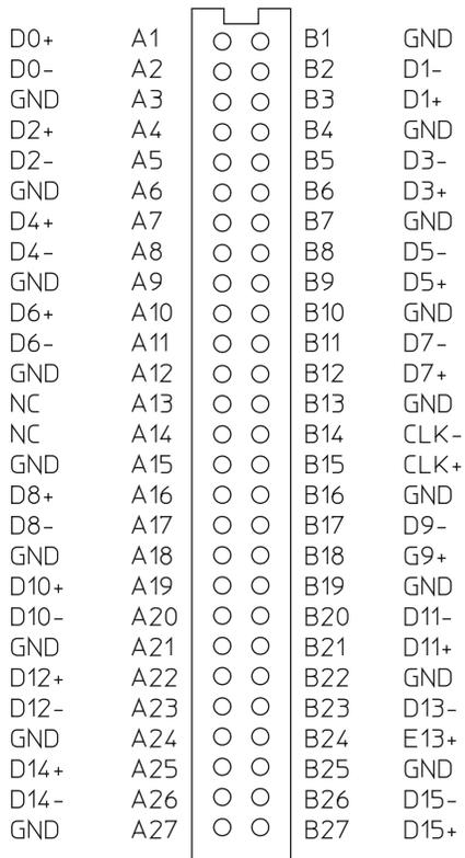
**Figure 8.9. Pad numbers for E5405A 17-bit differential probe.**
