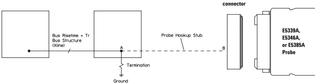
Figure 5.22. Agilent E5339A, E5346A, and E5385A design rules
