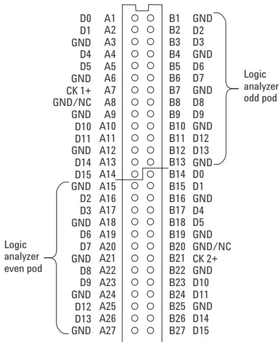
Figure 8.8. Pad numbers for E5404/06A 34-channel single-ended probes.
