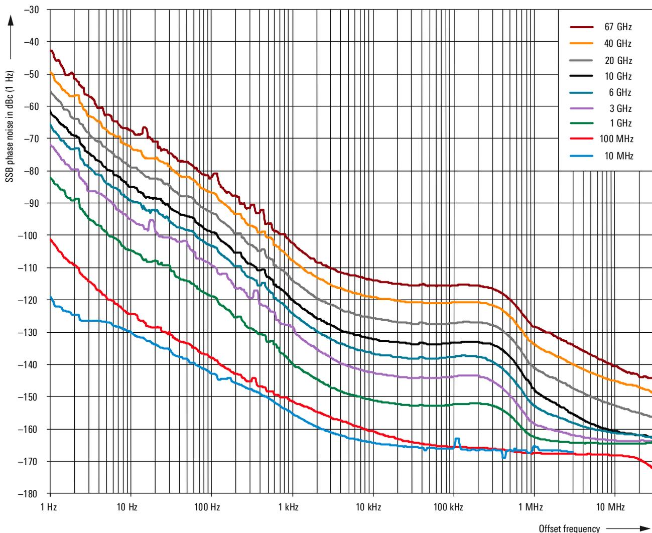
The ultimate solution is the R&S®SMAB-B711(N) ultra low phase noise option, which sets new standards with its exceptionally low phase and wideband noise across the entire offset range.
