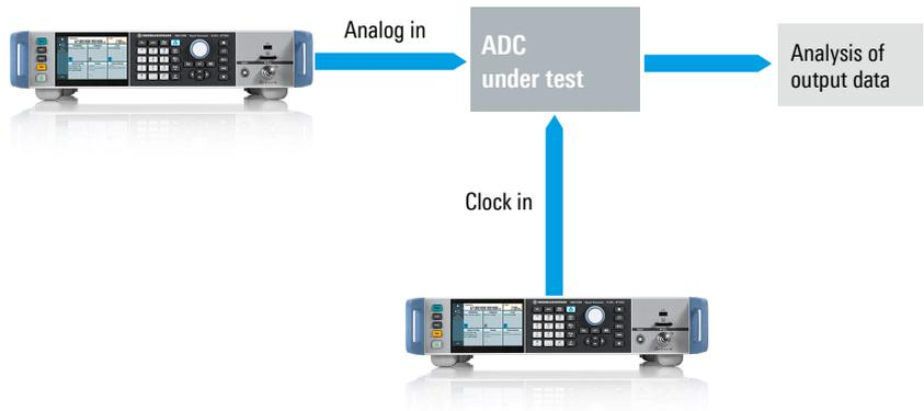
Compact ADC test setup for clock signals up to 6 GHz with a single R&S®SMA100B with an integrated second source
