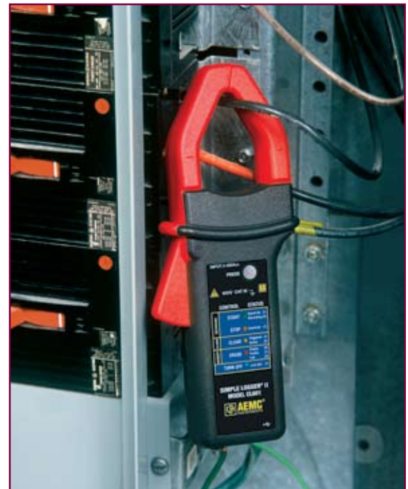
Easily log current in power panels.
