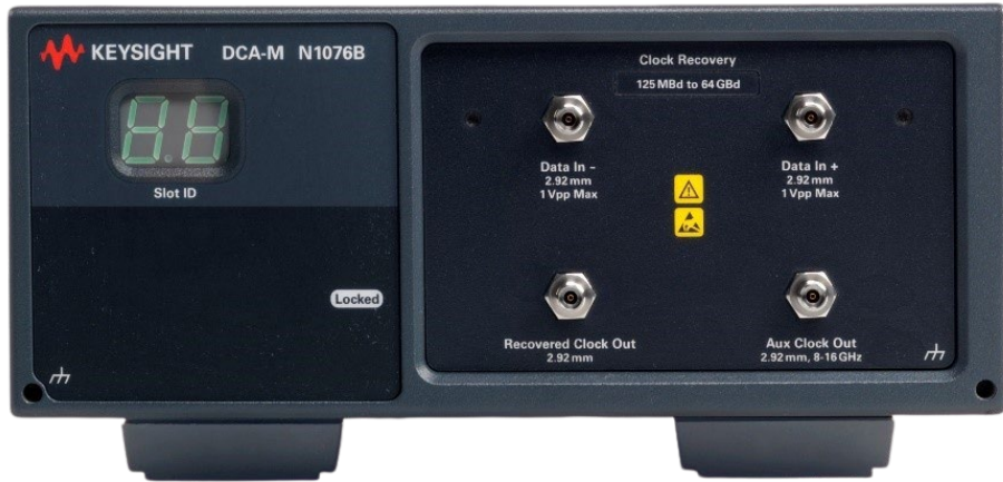
Figure 20. N1076B Electrical clock recovery with option 264
