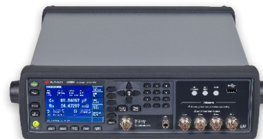
Keysight E4980A | Precision LCR Meter; 20 Hz to 2 MHz
