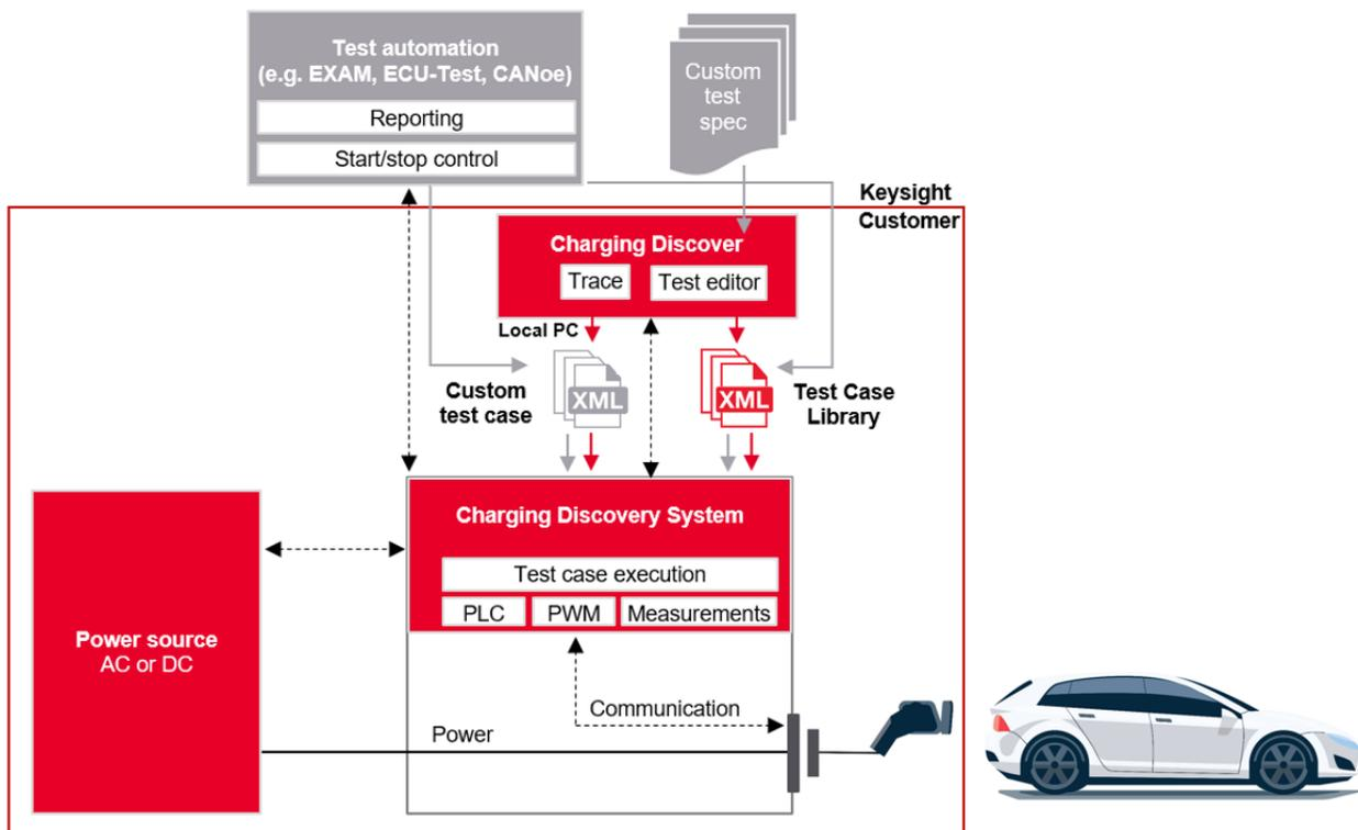
Figure 6. Interface topology of CDS with Expert mode.
