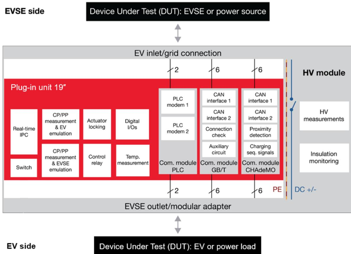
Figure 2. Block diagram of CDS architecture.
