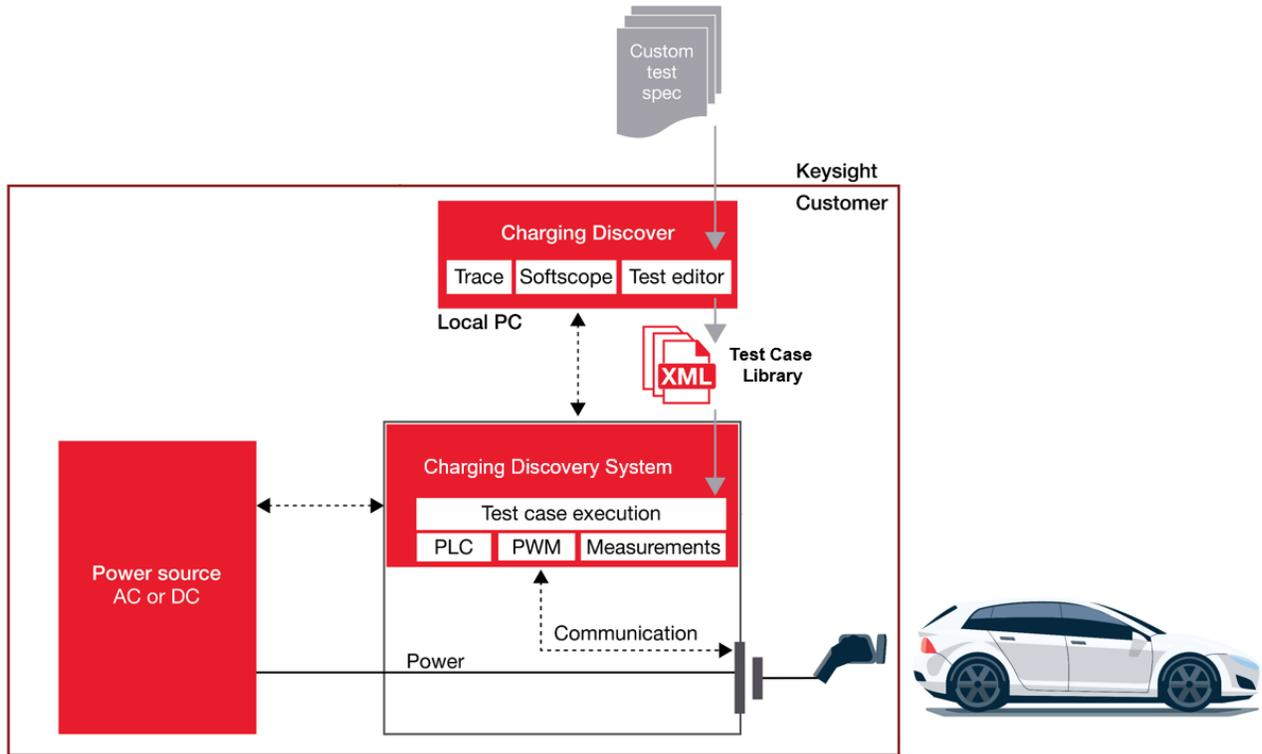
Figure 5. Interface topology of CDS with basic functionality.
