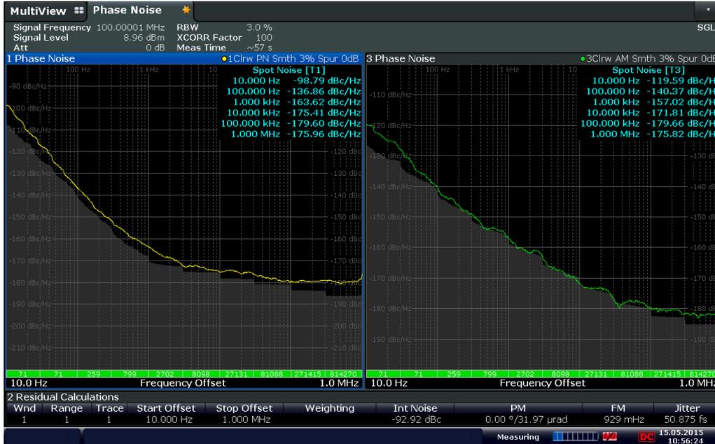
The R&S®FSWP can measure phase noise and amplitude noise simultaneously. The results can be displayed in separate windows or together in one window (gray area: correlation gain of the R&S®FSWP, green trace: amplitude noise, yellow trace: phase noise).
