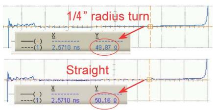
Less than 1% impedance change for bent cable
