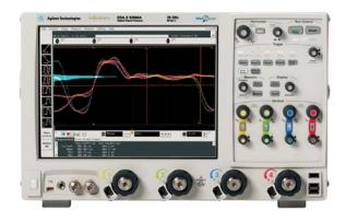
Use an Agilent Infiniium DS090000 or DS0X90000 Series oscilloscope with a W2641A TPA for DisplayPort source validation.
