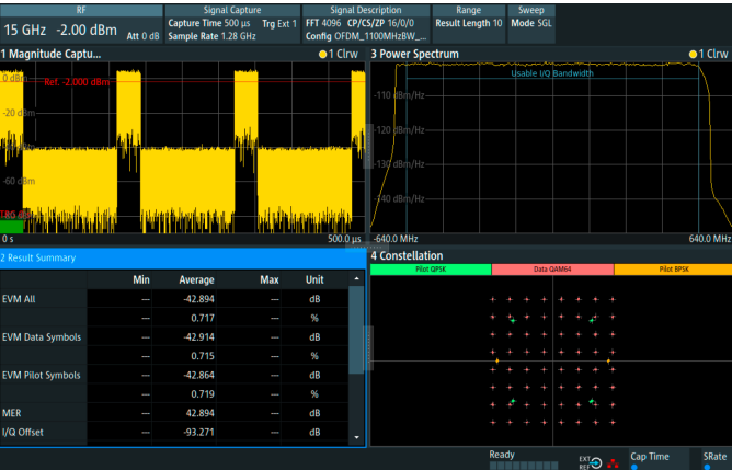
Analyzing a custom OFDM signal with 1100 MHz bandwidth
