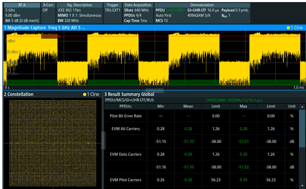
Analysis of a 4096QAM modulated 320 MHz wide IEEE 802.11bn signal
