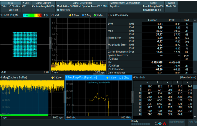
Analysis of a 1024QAM modulated signal: constellation diagram, result table, symbol table, EVM versus symbol and equalizer frequency response
