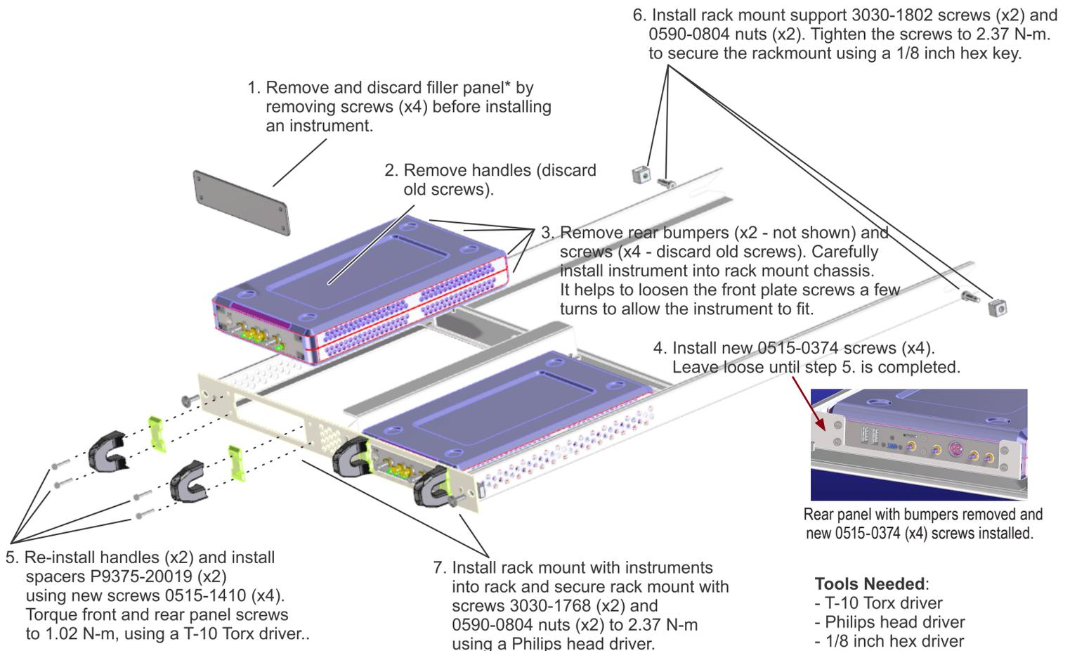
Installation of 1-High Rack Mount with Two Instruments
