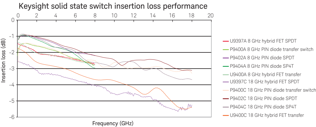
Figure 9. Keysight solid state switches—typical insertion loss performance
