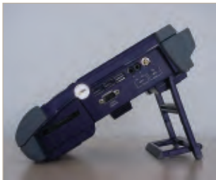
Figure 3: View of the right panel showing the CF card, RS-232, T1 Bantam, and ECL/NRZ ports
