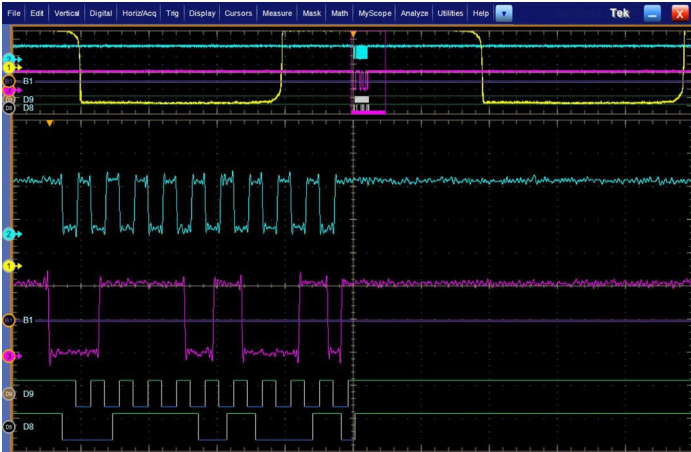
Integrated Logic Channels – Provide time-correlated analog and digital visibility for system debugging.
