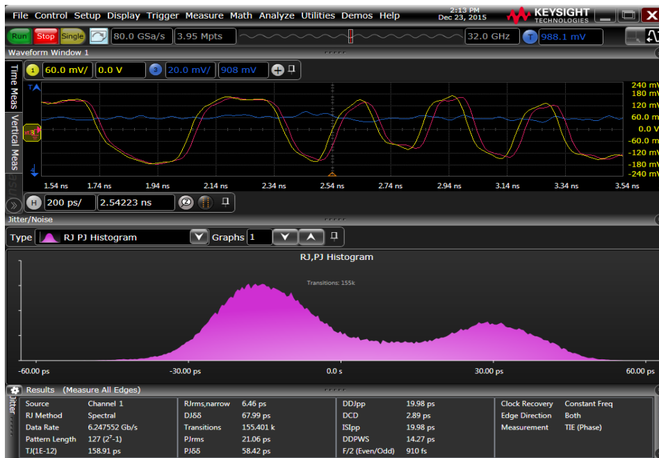
Figure 12. Jitter analysis results using EZJIT, showing the large amount of jitter in the original serial data waveform.
