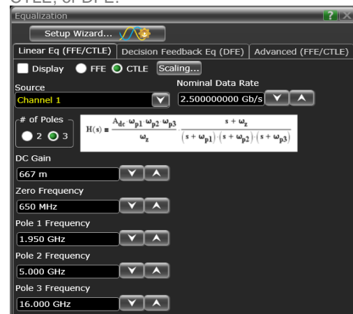
Figure 5. Serial data equalization supports both 2- and 3-pole CTLE.
