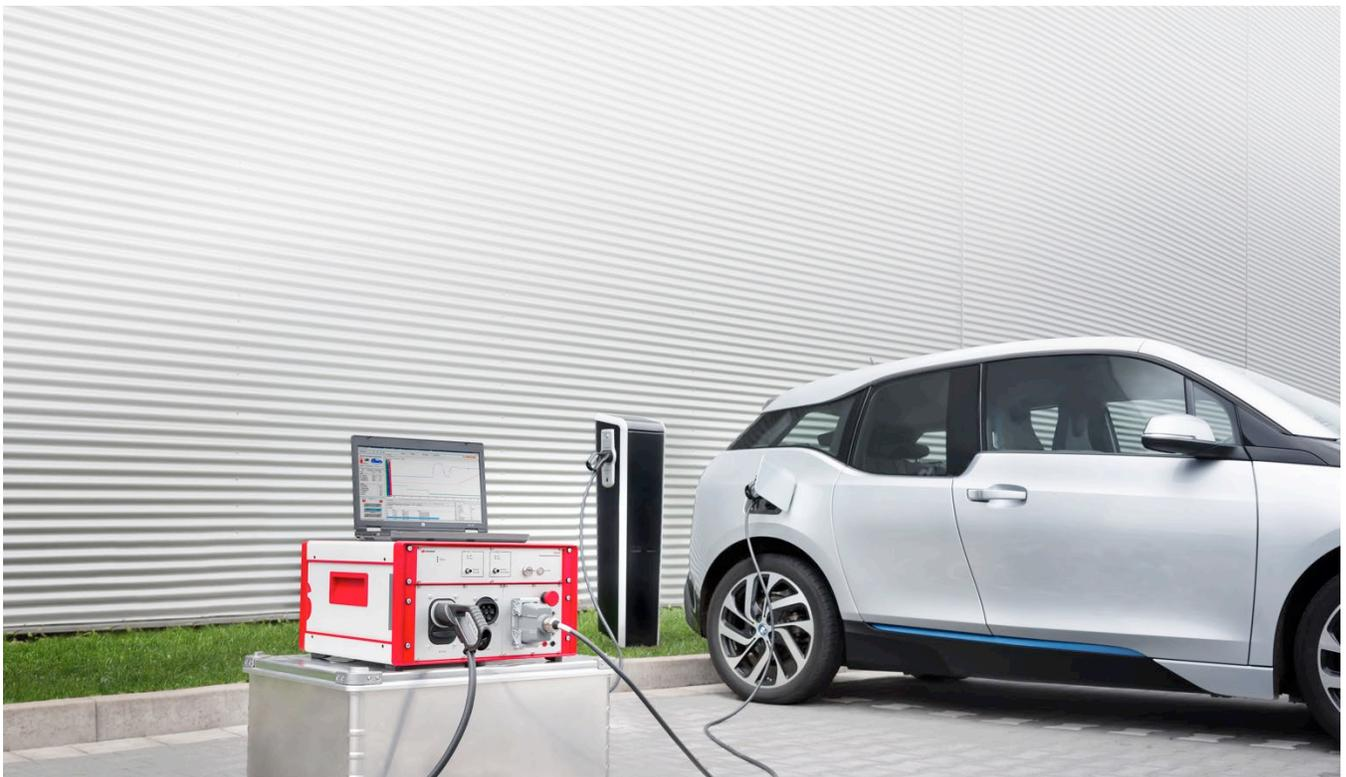
The Charging Discovery System used in the field as a man-in-the-middle system
