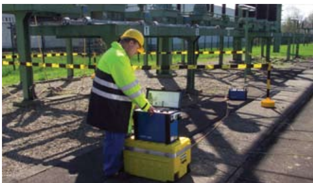
Measurement with CPC 100 and CP CU1
