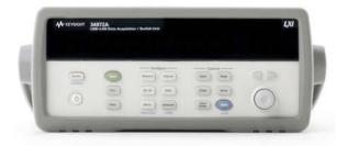
The Keysight 34970A data acquisition/data logger switch unit consists of a three-slot mainframe with a built-in 6 1/2 digit digital multimeter. Each channel can be configured independently to measure one of 11 different functions without the added cost or hassle of signal-conditioning accessories.
