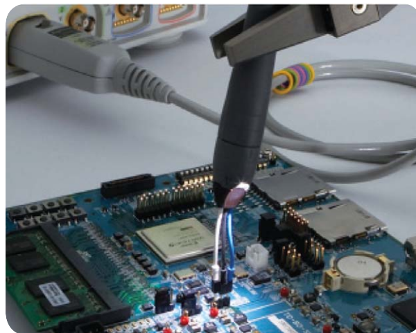
InfiniiMode probe with either socketed tip or solder-in tip allows convenient measurements of differential, SE and CM signals with a single probe. Probe head light is built in.
