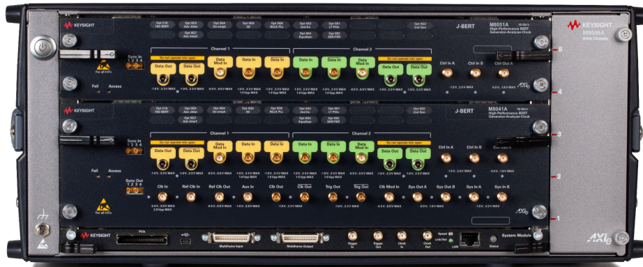
Figure 5. J-BERT M8020A high-performance BERT for accelerated receiver characterization. The configuration shows a 4 channel 16 Gb/s BERT in a 5-slot AXIe chassis consisting of one M8041A module with two BERT channels and clock synthesizer and one M8051A extender module with two additional BERT channels.
