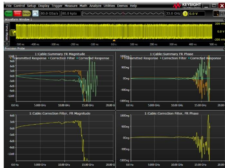
Figure 10. The magnitude and phase response of a cable corrected using PrecisionProbe.
