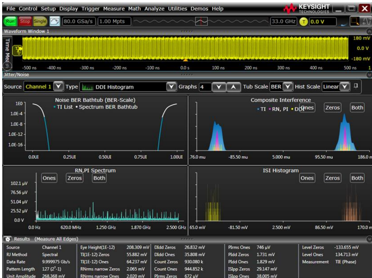
Figure 13. Noise analysis with EZJIT Complete software for insight into the sources of noise in the signal.
