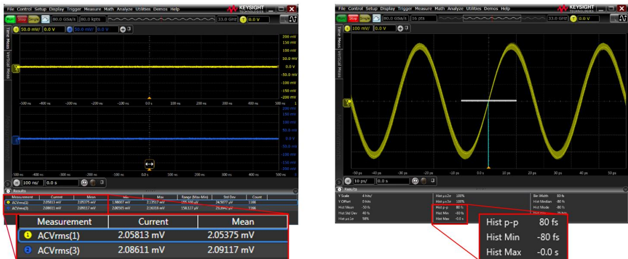
Figure 2. Infiniium V-Series ultra-low noise at 33-GHz full bandwidth and Jitter measurement floor of less than 100 fs (80 fs with 30 GHz input sine wave).
