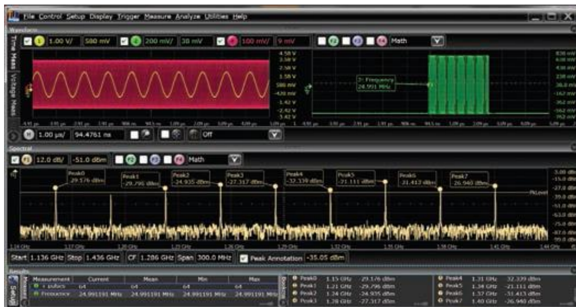
Figure 20. Peak search capability makes Infiniium Offline a frequency domain tool
