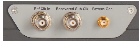
Figure 6. External reference clock input is one of the methods to enable SSC tracking by the hardware serial trigger.
