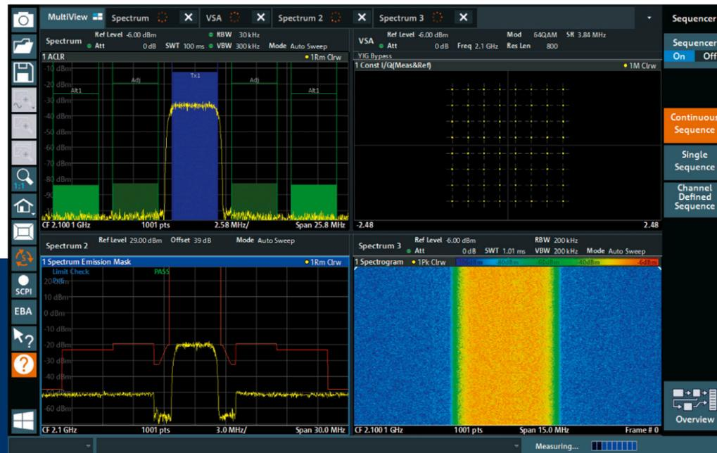
In many cases, the event based actions dialog eliminates the need for an external PC. Instead of SCPI programming, IF-THEN commands are set up via the GUI.
