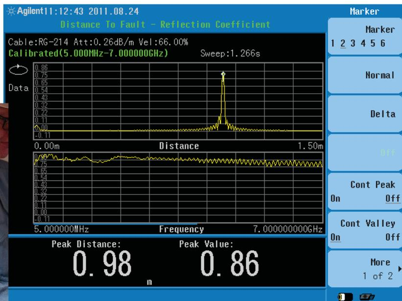
Optional cable and antenna test function offers a built-in VSWR bridge to measure cable loss, return loss, and distance-to-fault (exclusive to the N9342C HSA)
