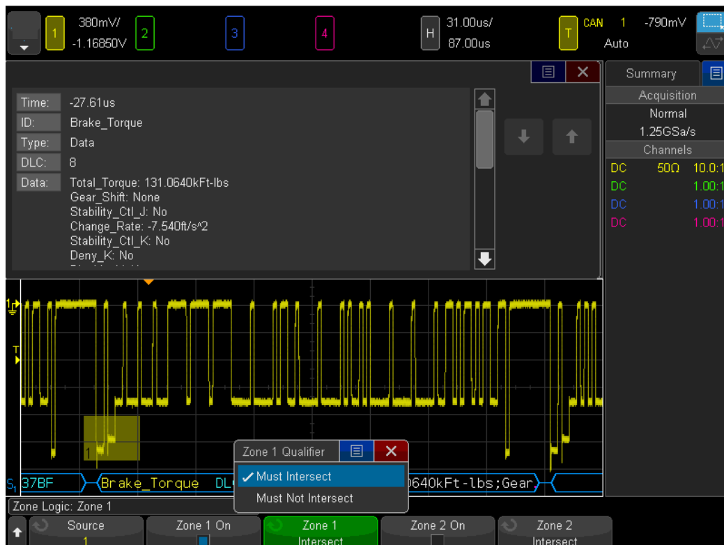
Figure 1. Capturing CAN bus arbitration while decoding CAN messages symbolically.
