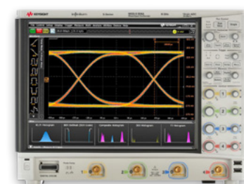
Keysight MSOS804A | Infiniium S-Series Digital Oscilloscope; 4-Channels, 8 GHz
