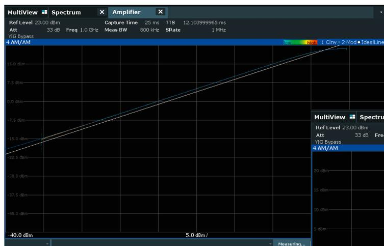
Gain transfer curve measurement (AM/AM) of an amplifier. For the curve above, a CW signal with a linear power ramp has been used as the stimulus. As expected, the AM/AM curve is a line. The curve on the right was measured using a digitally modulated signal generated by the R&S®SMW200A. The AM/AM is a cloud-like curve; the line width is due to amplifier memory effects.
