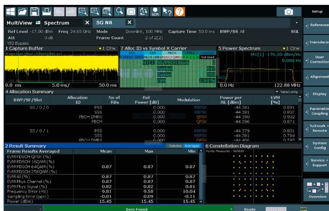
The R&S®FSW-K144 and R&S®FSW-K145 support all specified 5G signal bandwidths from 5 MHz to 400 MHz, with multiple numerologies, multiple bandwidth parts and modulation formats from QPSK to 256QAM.
