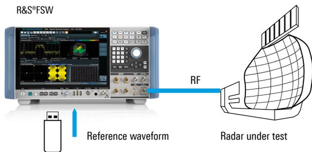
The analyzer shows trends and performs statistical analyses on all pulse, chirp and hop parameters. Trend analysis allows you to quickly identify the effects of supply voltages (or their frequencies, such as 50 Hz or 400 Hz) and to rapidly verify frequency hopping patterns and changes in the pulse repetition interval.
