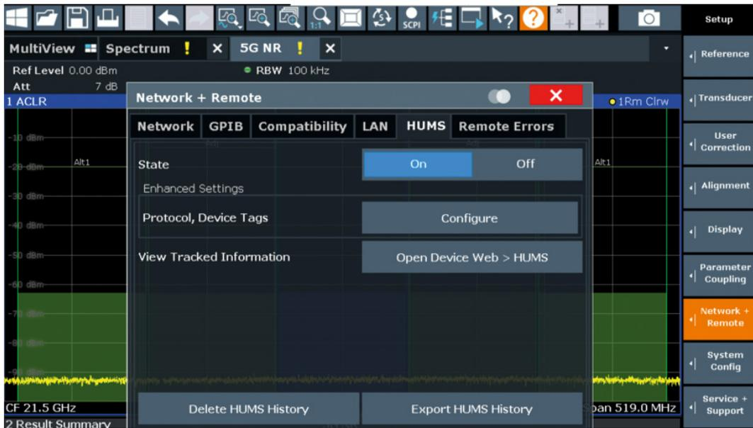
The R&S®FSW-K980 HUMS option provides utilization and health data via SNMP or REST interfaces
