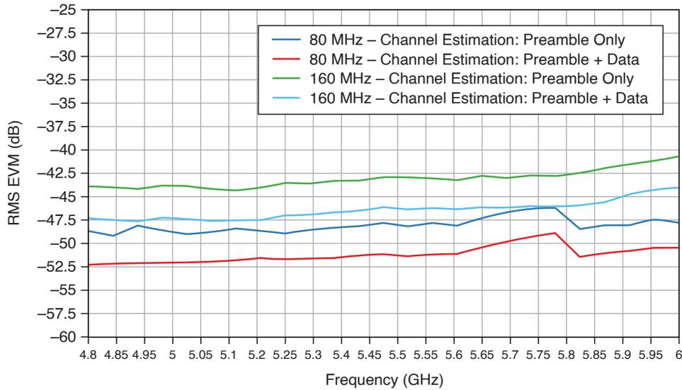
Conditions: RF output loopback to RF input; Offset Mode: Enabled; MCS index: 9; RF output average power: 0 dBm; Reference level: average power + PAPR; Internal LO
