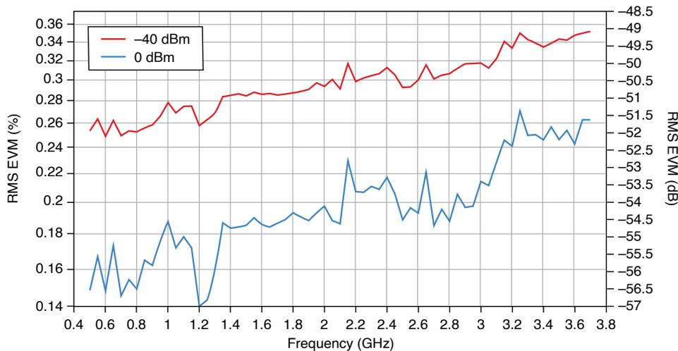
Conditions: RF Output loopback to RF Input; Offset Mode: Enabled; Independent onboard LOs; 20 MHz BW, Uplink, FDD; Average power + PAPR
