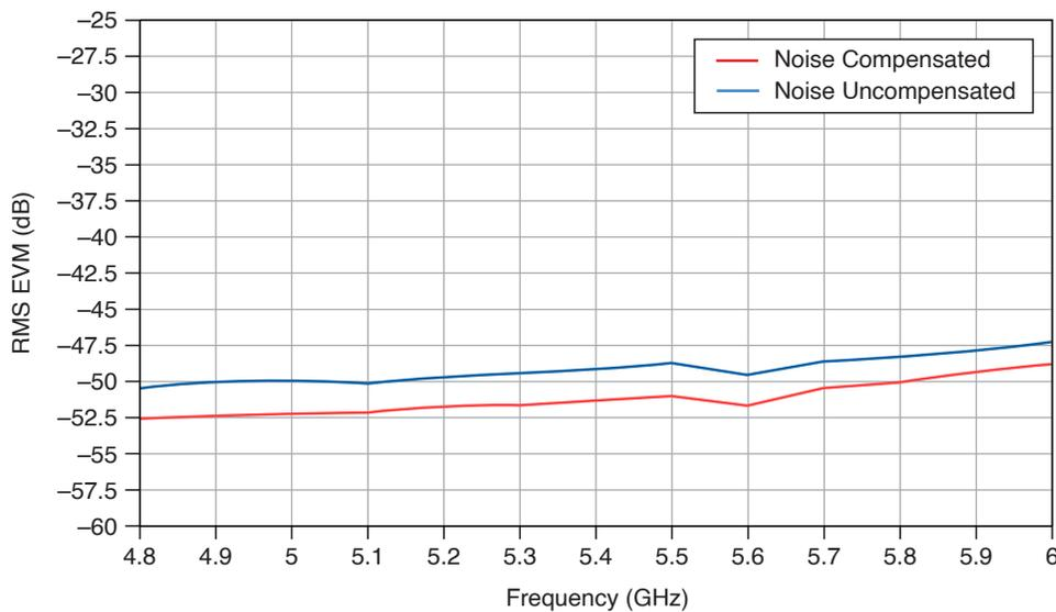
Conditions: RF output loopback to RF input; Waveform bandwidth: 80 MHz; MCS index: 11; Offset Mode: Enabled; RF output average power: -15 dBm; Reference level: average power + PAPR
