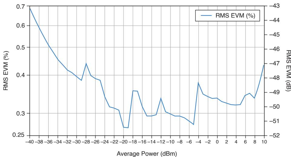
Conditions: RF output loopback to RF input; Reference/power level: average power +PAPR; Waveform bandwidth: 100 MHz; Subcarrier spacing: 30 kHz, uplink, 256 QAM; Offset Mode: Enabled; Reference Level Headroom: Default (1 dB); Measurement length : 3 slots
