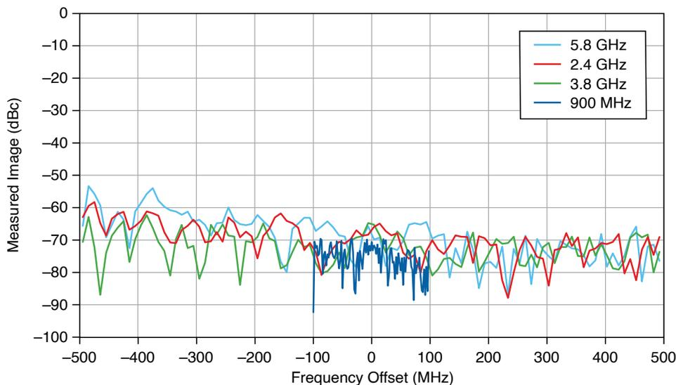
**Figure 10.** Input Residual Sideband Image, -30 dBm Reference Level, Measured
