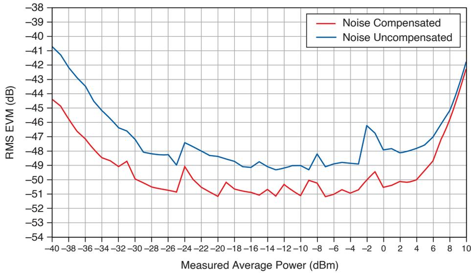
Conditions: RF output loopback to RF input; Waveform bandwidth: 80 MHz; MCS index: 11; Offset Mode: Enabled; Carrier frequency: 5.5 GHz
