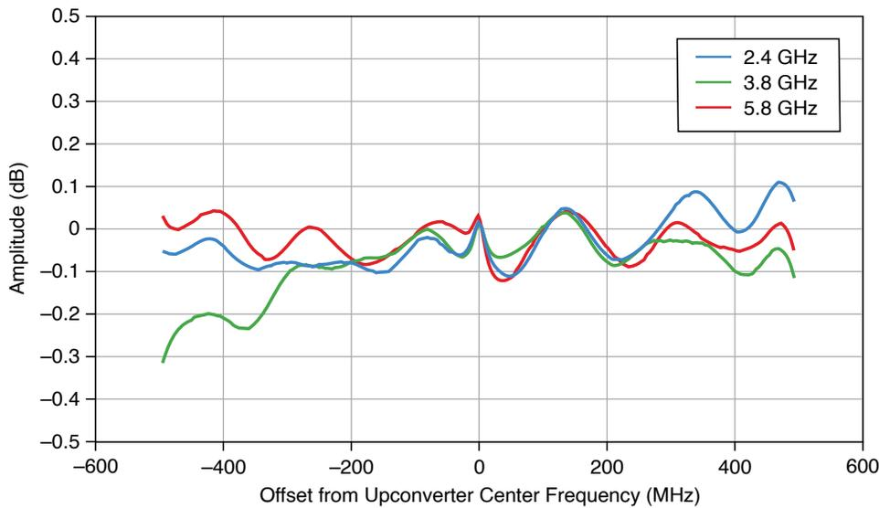
**Table 25.** Output Frequency Response (dB), Equalized (Offset Mode is Enabled)
