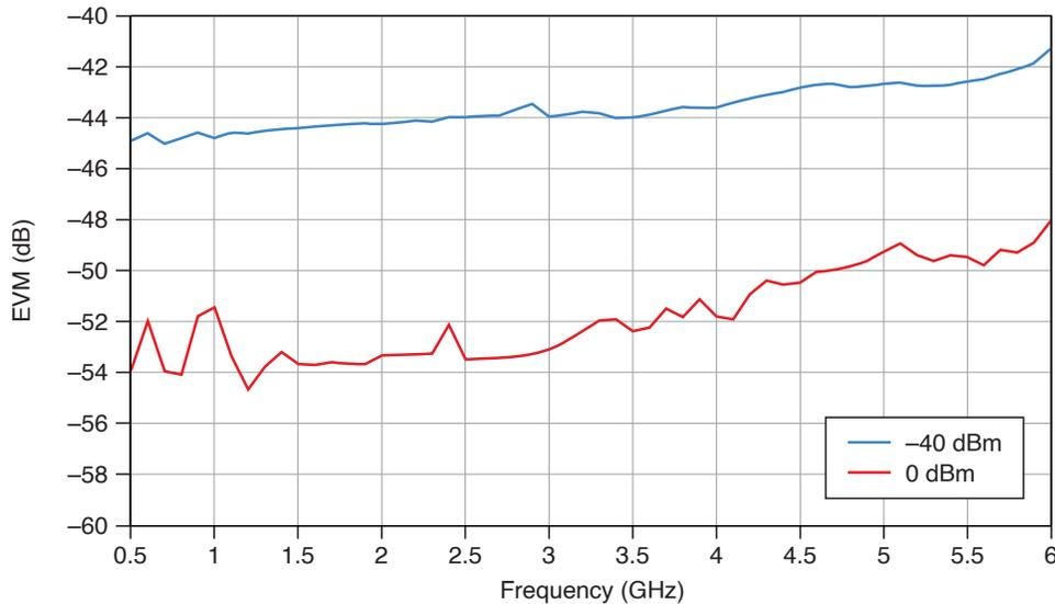
Conditions: 20 MHz bandwidth 64-QAM modulated signal. Pulse-shape filtering: Root-raised cosine, alpha=0.25; PXIe-5841 RF Input reference level, RF output peak power level set to value specified in legend; Offset Mode: Enabled; Reference Clock source: Onboard; Acquisition length: 300  $\mu$ s
