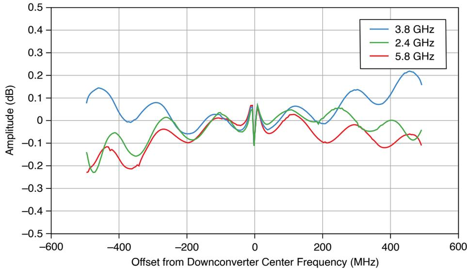
**Table 15.** Input Frequency Response (dB), Equalized (Offset Mode is Enabled)
