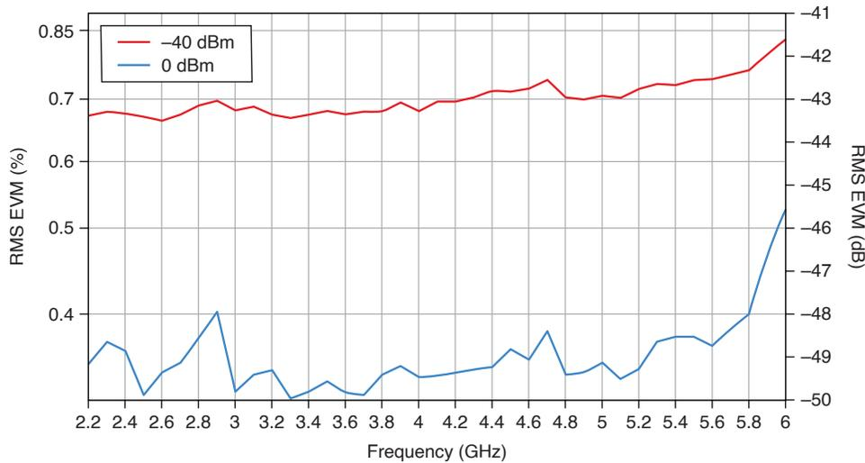
Conditions: RF output loopback to RF input; Waveform bandwidth: 100 MHz; Subcarrier spacing: 30 kHz, uplink, 256 QAM; Offset Mode: Enabled; Reference Level Headroom: Default (1 dB); Measurement length: 3 slots
