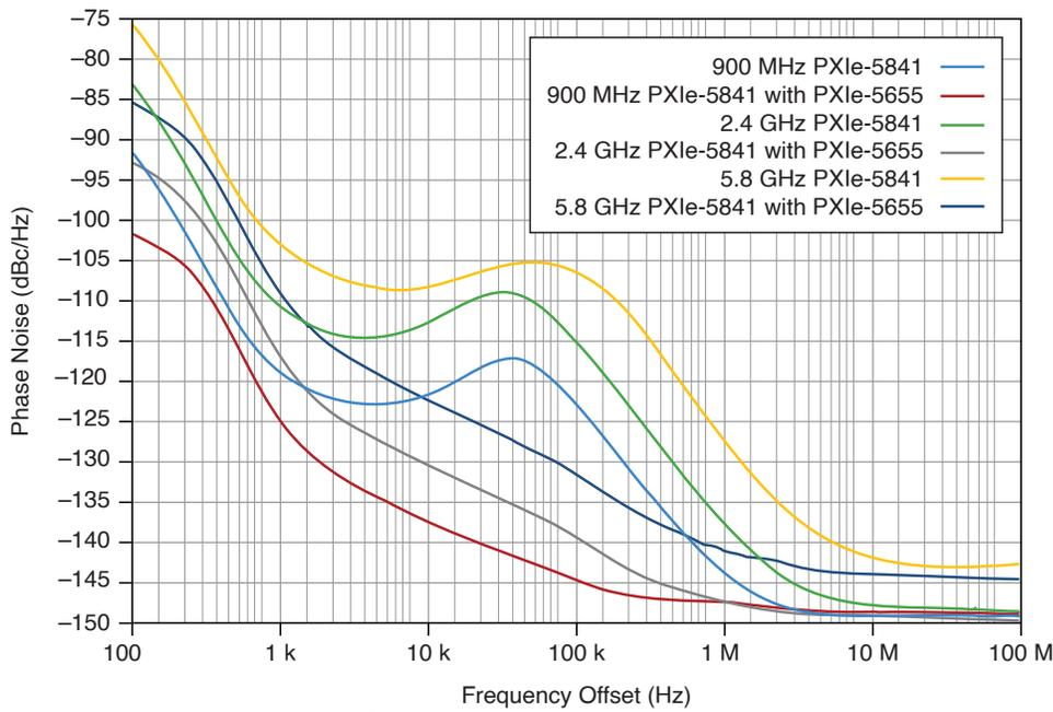
Conditions: Measured Port: RF OUT; Reference Clock: Onboard; Spurs not shown.
