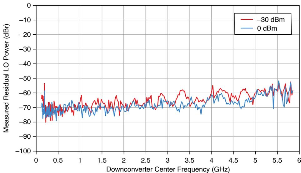
**Figure 8.** Input LO Residual Power, Measured (PXIe-5841 with PXIe-5655)
