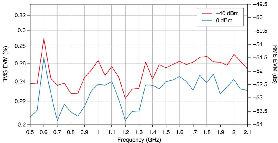
Conditions: RF output loopback to RF input; Offset Mode: Enabled; Independent onboard LOs.
