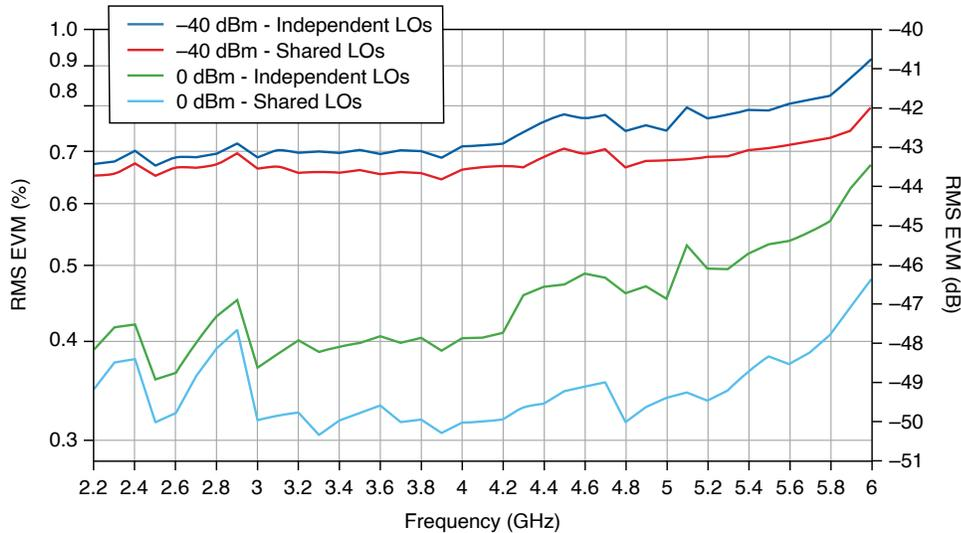
Conditions: RF output loopback to RF input; Waveform bandwidth: 100 MHz; Subcarrier spacing: 30 kHz, uplink, 256 QAM; Offset Mode: Enabled; Reference Level Headroom: Default (1 dB); Measurement length: 3 slots
