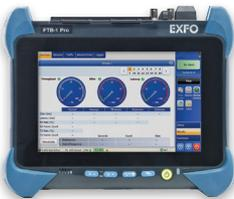
**EXFO FTBx-88260-FR1** | RF Spectrum Analyzer; 450 MHz to 6 GHz with RTSA
