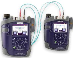
**Viavi Solutions OLTS-85P-35** | Quadmode Tier 1 Optical Loss Test Kit with Patch Cord Microscopes
