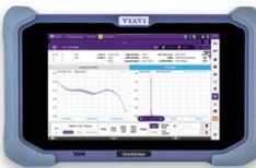
**Viavi Solutions SPA06MA** | RF Spectrum Analyzer; 9 kHz to 6 GHz
