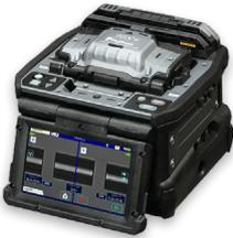
**Fujikura (AFL) 90S+** | Core Alignment Fusion Splicer
