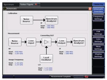
The R&S°FSV-K30 option expands the R&S°FSV or R&S°FSVA signal and spectrum analyzer by adding measurement functionality otherwise only provided by special noise measurement analyzers.
