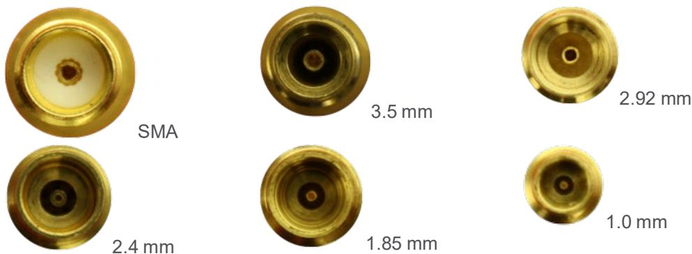
Figure 26. Typical female input connectors
