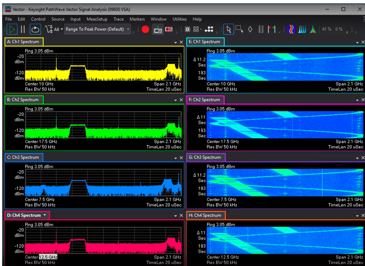
Figure 1. Software such as PathWave Vector Signal Analysis (VSA) for EW helps you identify and log key metrics for pulse-modulated radar signals in aerospace, defense, and EW.
